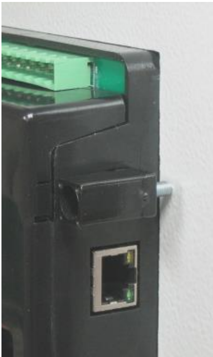
Installation of screw type bracket
