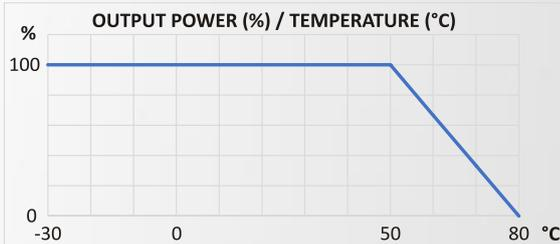
Thus if the charger is forced to operate in an environment above +50°C, it will simply reduce its output power to the corresponding value in the above chart and continue normal operation.
